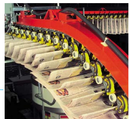
Application sample: Insertion system for regionalization and supplementation of newspapers (© FERAG AG)
