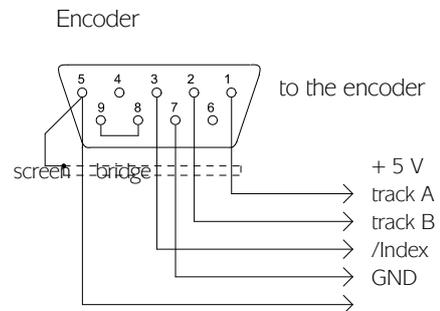
The precise allocation of the encoder jack and the significance of the signals (temporal trends and interrelationships) can also be found in the hardware reference section.
